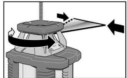
When working with the remote control, this must be oriented to the laser's operating field.
