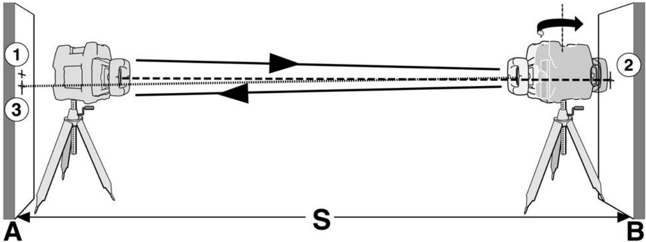
Two parallel wall surfaces at least 10m ( or 50 ft) apart are required for the vertical check.
